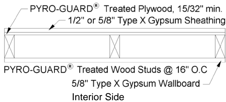
FIGURE 4—1-HOUR FIRE-RESISTANCE-RATED EXTERIOR WALL ASSEMBLY Use where wall is required to be fire-resistance-rated from the exterior and interior sides. (ESR-1791 1-HR)
